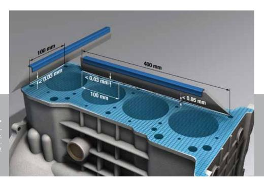
Maximum values for component unevenesses and distortions for passenger cars. Practical measurement using a straightedge and the light-gap method.
