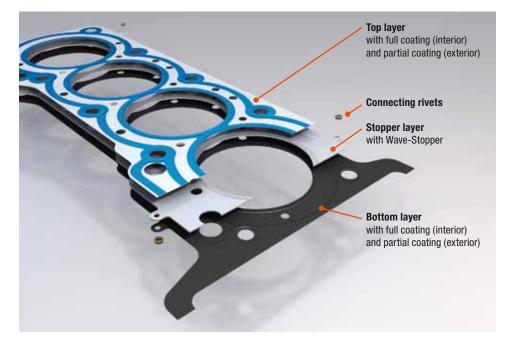
layer steel head gaskets. For improved sealing of gases and liquids, beads around combustion chambers and oil/coolant passages increase the local sealing pressure (macro sealing), whilst full-surface or partial elastomer coatings provide additional sealing tightness (micro sealing).
